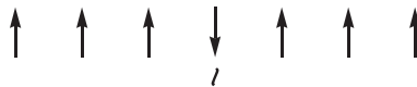
Figure 23.2 A single local spin-flip excitation of a ferromagnetic system. The resulting state is not an eigenstate of the Heisenberg Hamiltonian.
